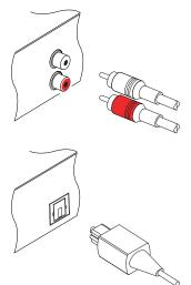
You will need to obtain an audio cable (RCA cable) to connect the audio connectors. Plug one end of the cable into the AUDIO L (white) and AUDIO R (red) sockets on the digital receiver, and plug the other end into the matching sockets on your television or audio system.
